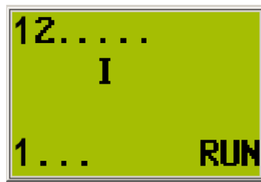
Figure 1-4. Programmable Logic Controller status display.
