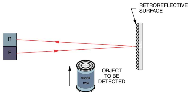
Figure 12. Retroreflective sensing.
