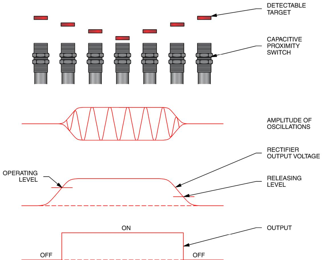
Figure 18. Operation of a capacitive proximity sensor.
