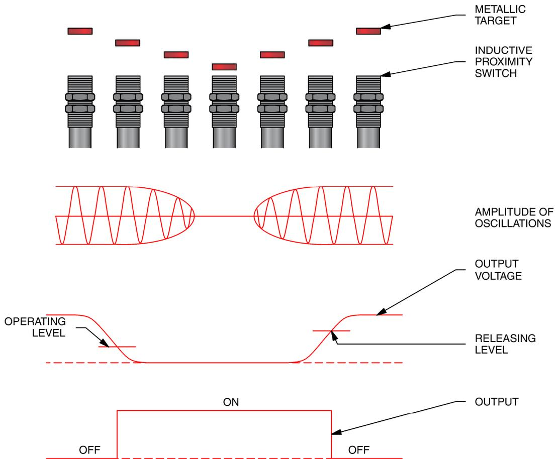
Figure 24. Operation of an inductive proximity switch.
