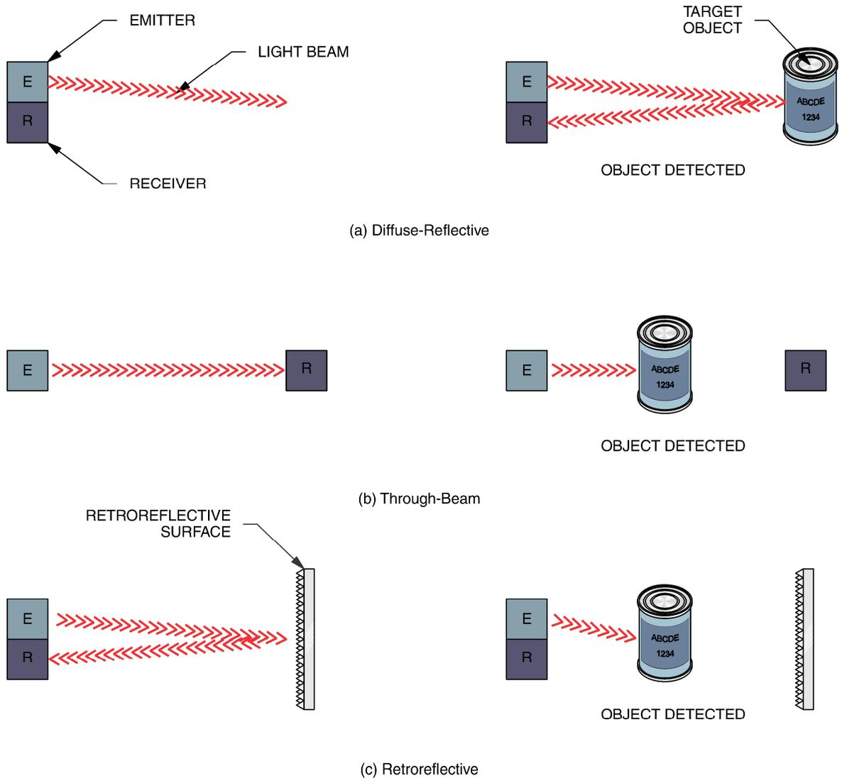
Figure 2. Photoelectric sensing modes.
