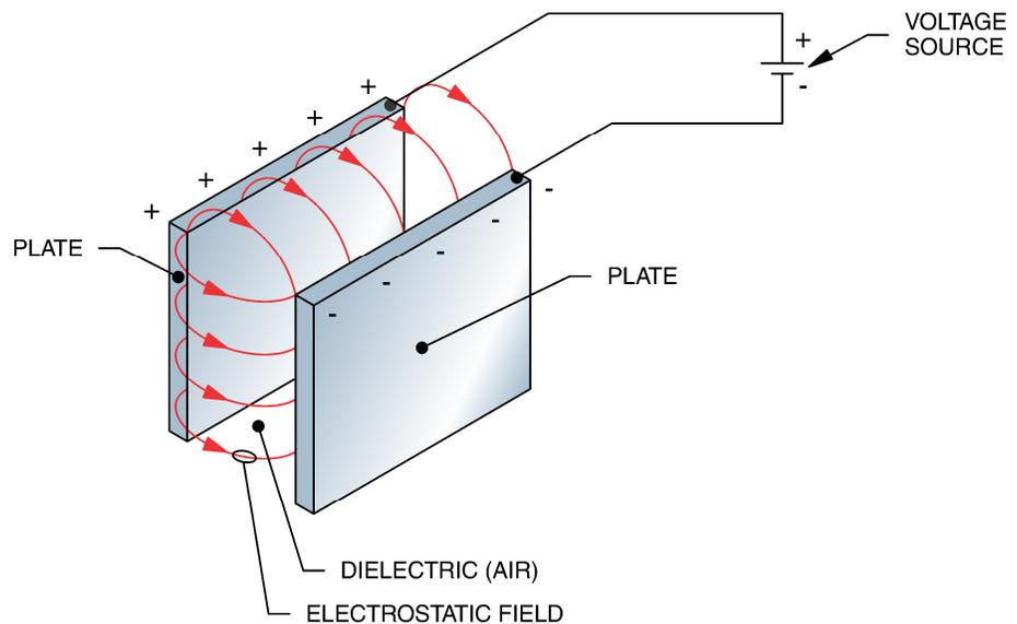
Figure 17. Charged capacitor.
