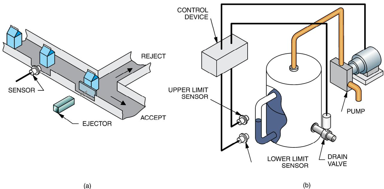
Figure 19. Sensing liquid level using capacitive proximity switches.
