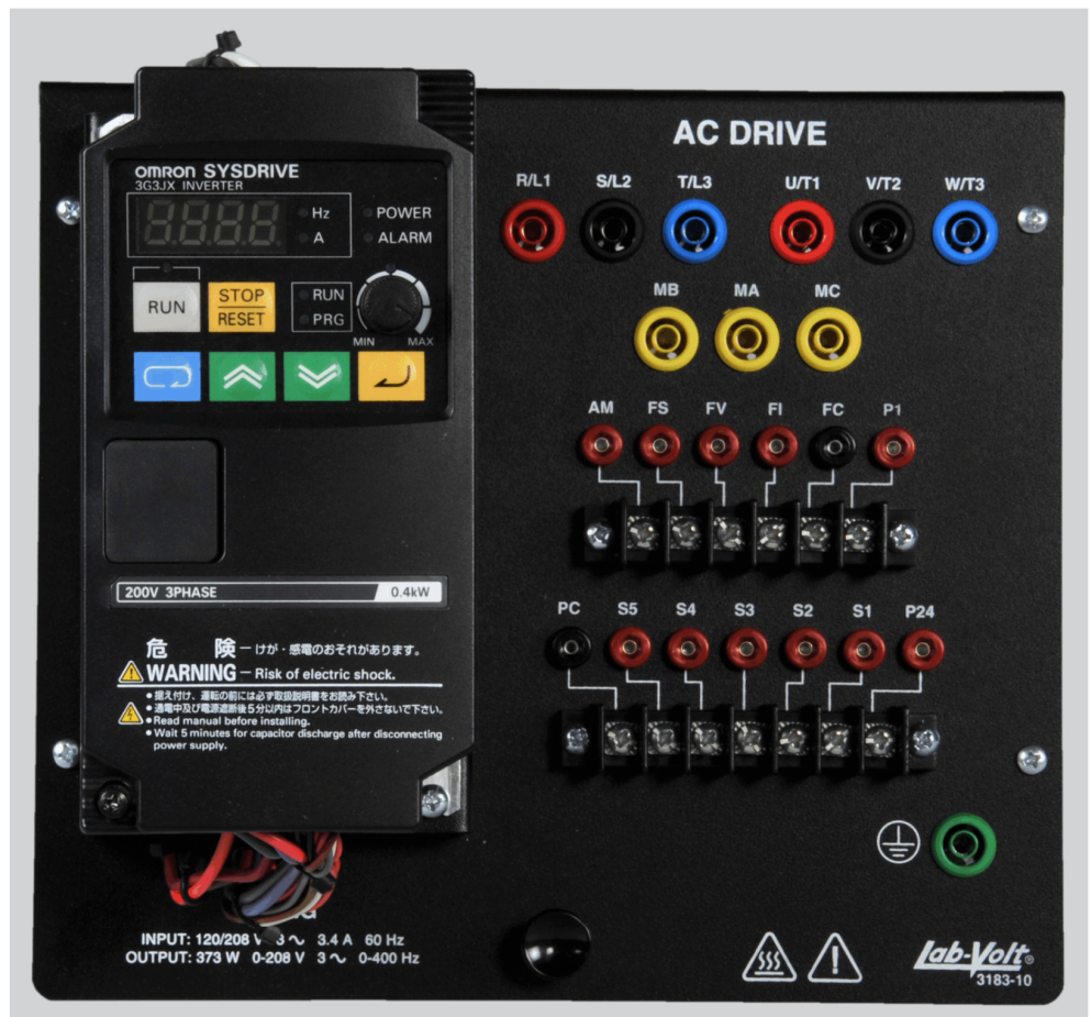
Figure 1-2. AC Drive, model 3183 (version 120/208 V, 60 Hz).
