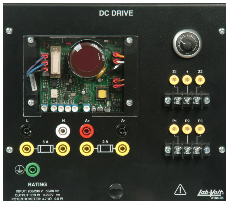
Figure 2-2. DC Drive module, model 3184-5 (version 208/230 V, 50/60 Hz).
