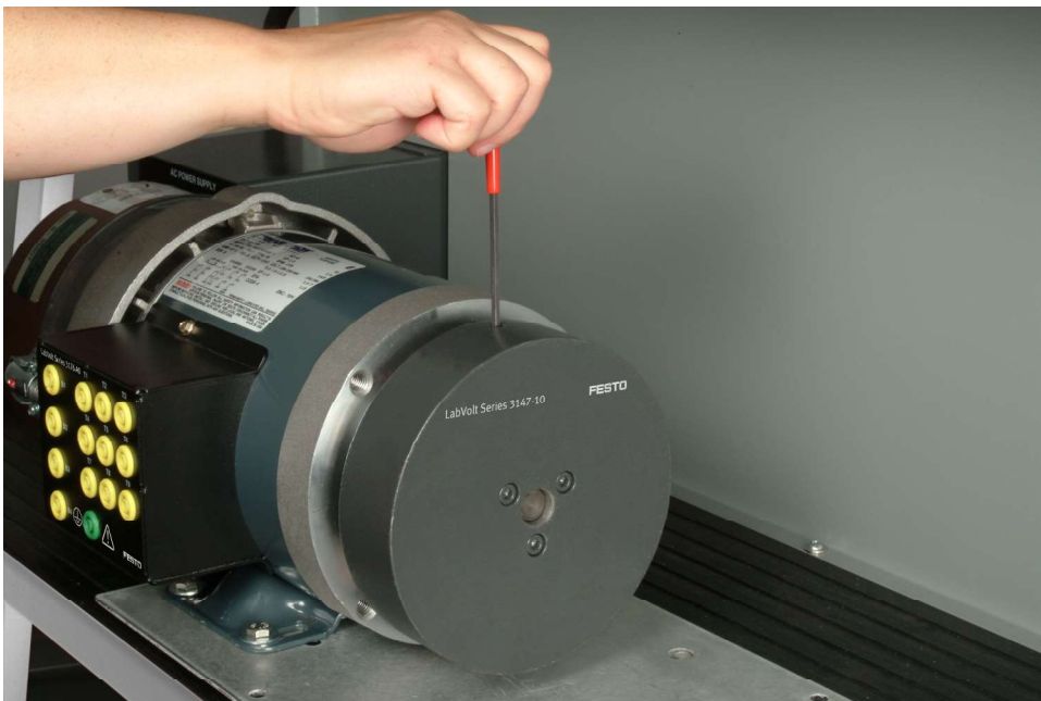
Figure E-3. Tighten the setscrew with a hexagonal key.
