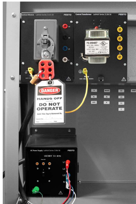
Figure D-4. Installation of padlocks and hasps.
