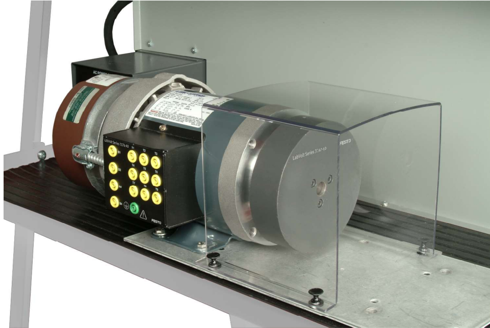
Figure E-4. Installation of the Safety Guard.
