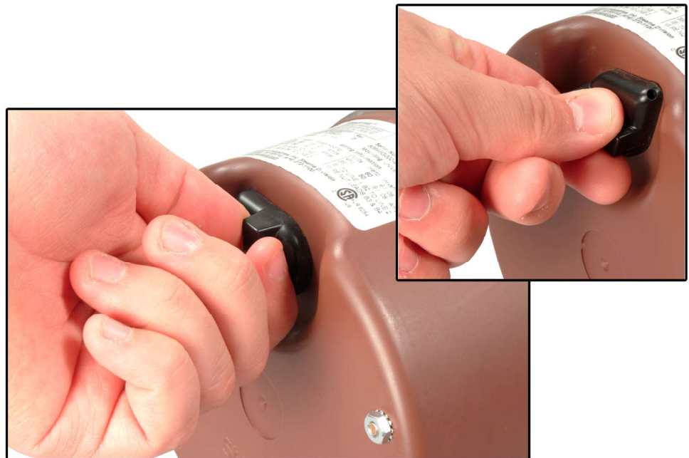
Figure 3-2. Release of friction brake on the Brake Motor.
