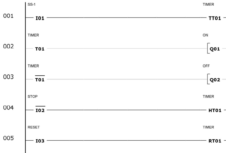
Figure 1-25. Ladder program of the PLC timing relay circuit.
