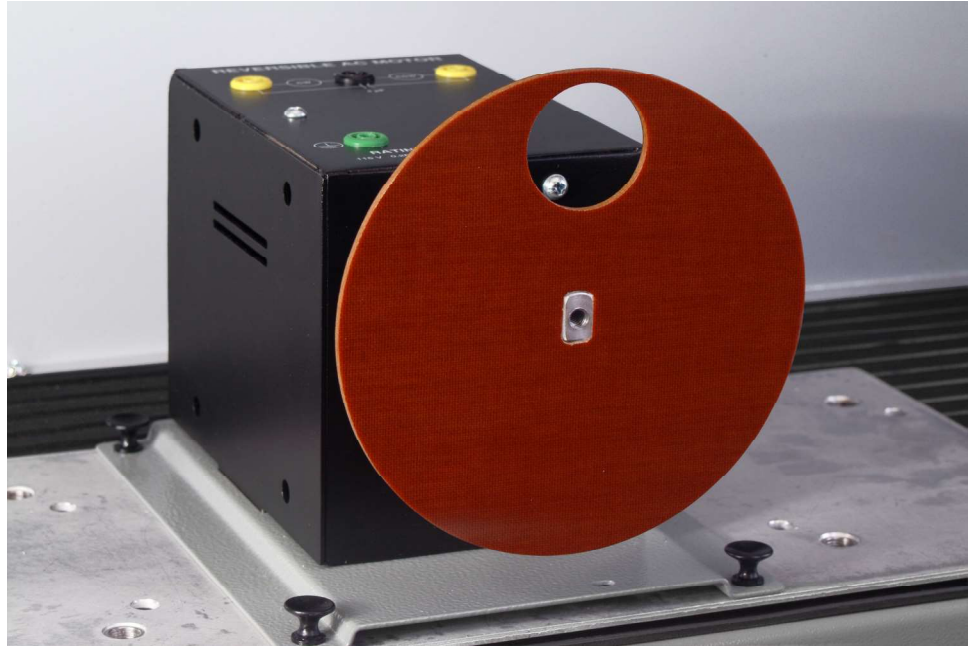
Figure 33. Align the opening in the center of the disk to fit the end of the bushing.
